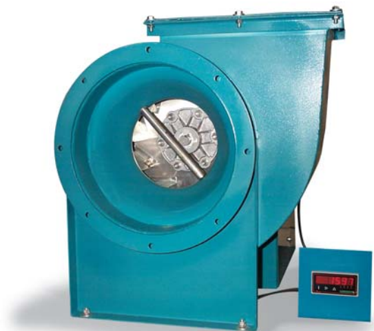
B. Fan operating with obstructed inlet produces 1597 CFM
